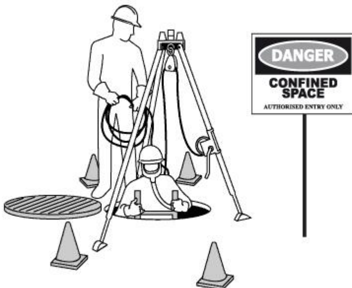
Figure 7: Standby person monitoring the confined space with rescue equipment and sign in place.
